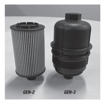
Vehicles equipped with the GEN-3 3.0L engine may encounter an illuminated Malfunction Indicator Lamp (MIL) if the oil filter cap is not tightened to 18 ft. pounds (221 inch pounds). Trouble code P0524 may also be stored in memory on the DT and JL vehicles due to an improperly tightened cap.
